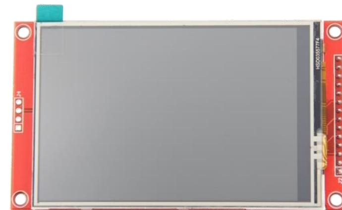
3.5" colour screen Capacitive touch panel Landscape format
